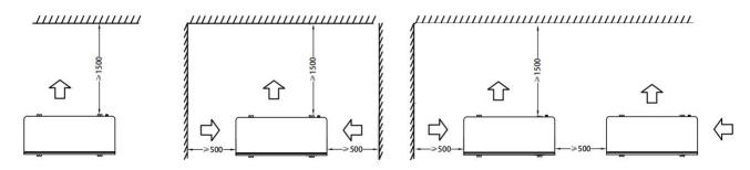
Do not put anything less than one meter in front of the heat pump.
