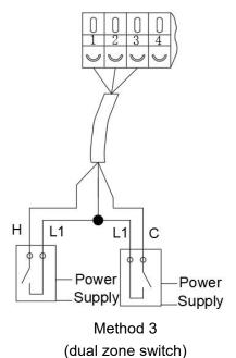
Voltage220-240VACMaximum Current0.2AWire Specifications20AWG/0.75mm²
