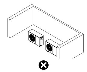
③ Do not install the unit vertically up and down. The condensate of the unit is discharged from the chassis. If the condensate of the unit drips onto the unit below, it will easily cause the unit below to freeze.
