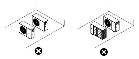
② Don't make the air inlet of the unit opposite to each other and don't make the air inlet of the unit blocked by the wall.
